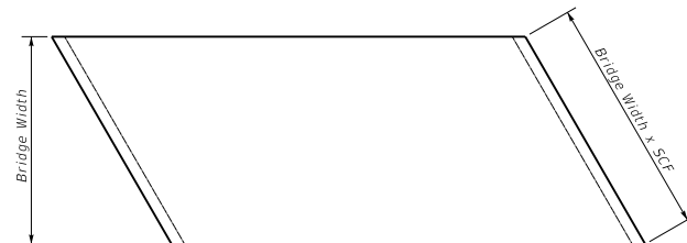
PLAN OF SUPERSTRUCTURE SLAB
